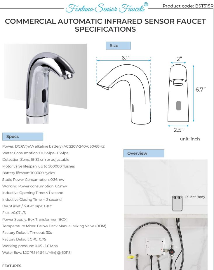
Commercial Grade Faucet, ADA Compliant, Cast Brass Spout, Quick Connect Fittings, Integrated Water Shut-off, Hygienic Line Flush, Water Usage and Battery Strength Reporting, Self-adapting Sensor
